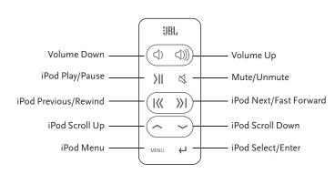
IBL 10-Button Remote Technical Specifications Transmission: Frequency: 38kHz Operating Range: 20 feet Battery Type: CR2025 3V Dimensions: Width: 1.29"(33mm) Height: 3.38" (86mm) Depth: o.23" (6mm) Weight (including battery): 1.2 OZ.
